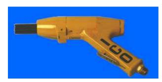
VARIOUS KINDS OF APPLICATION OF THE PNEUMATIC NEEDLE CHISEL, FOR SCALING ON IRREGULAR SURFACES.
